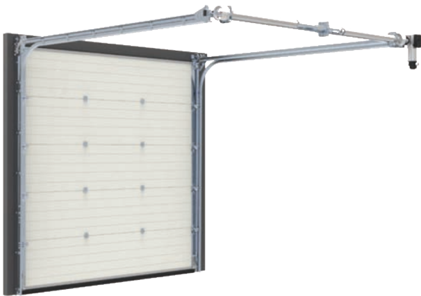
The bend on the guides has a radius that enables the door to be opened even with very low architraves (200 mm, 250 mm and 320 mm).
